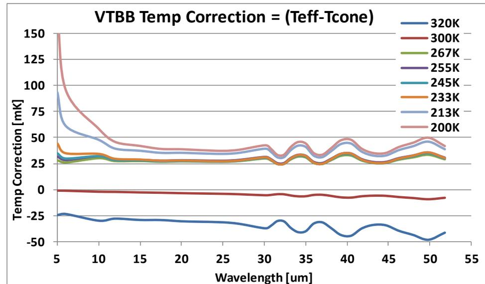
• IR CDS measurement of target radiance requires accurate knowledge of the blackbody (BB) radiances: (1)  $L_{bb}(\lambda, T_{bb}) = \varepsilon_{bb}P(\lambda, T_{bb}) + (1 - \varepsilon_{bb})P(\lambda, T_e)$
