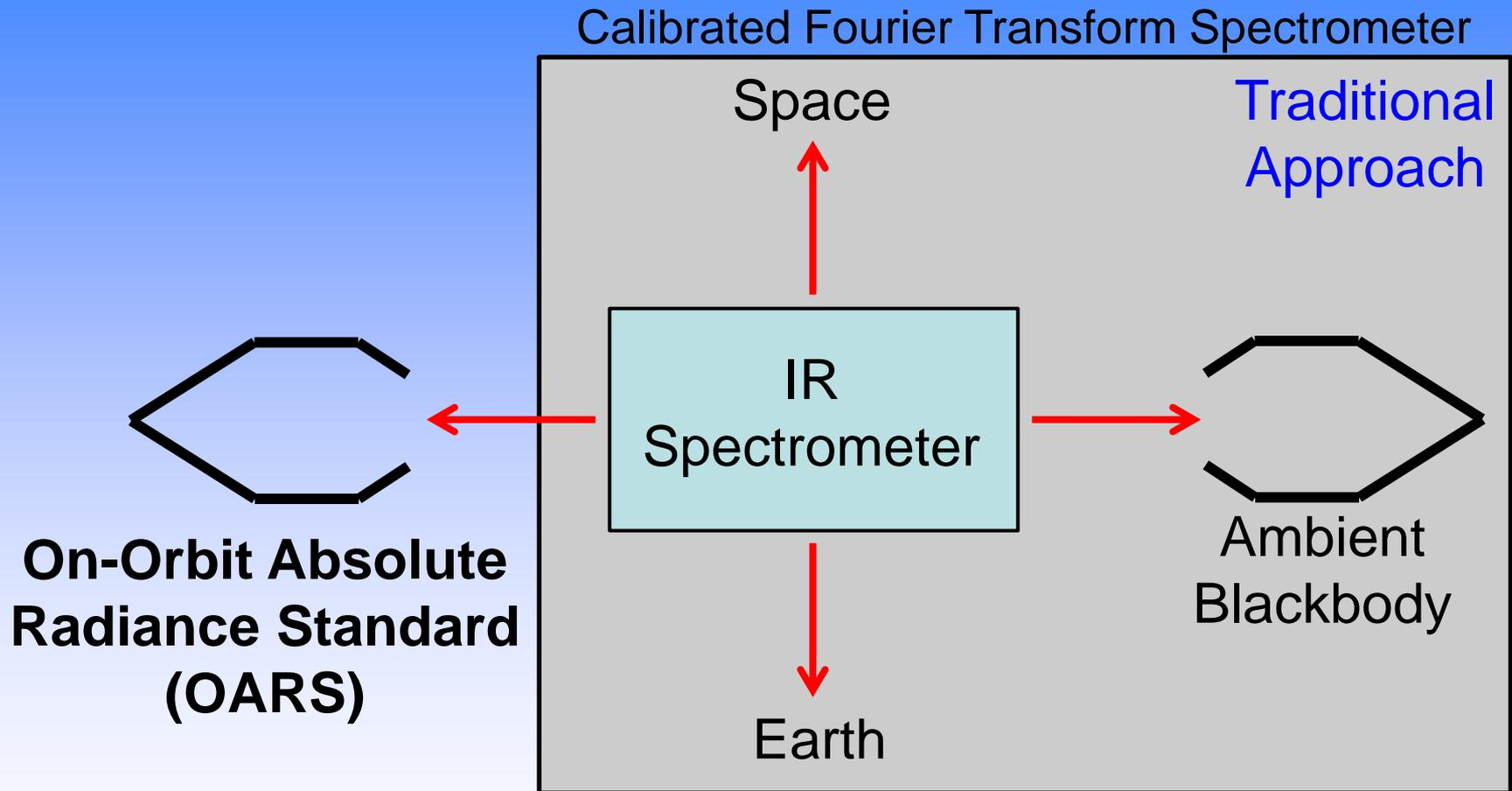
OARS Provides End-to-End Calibration Verification On-Orbit
