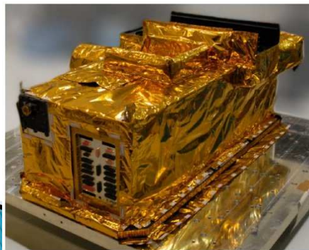
Engineering model of SGLI-IRS for vibration test configuration
