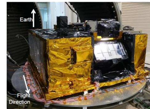
Engineering model of SGLI-VNR for thermal vacuum test configuration
