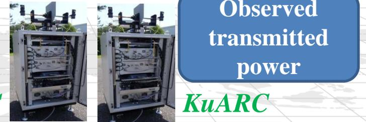
To calibrate the received power and the transmitted power of DPR, the difference between observed power and estimated power is evaluated.
