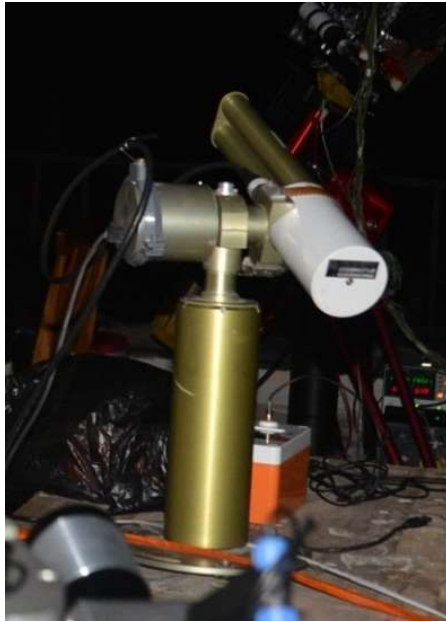
Lidar and CE-318- Lunar for day-night aerosols optical depth
