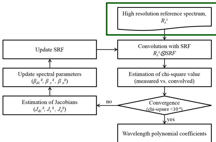
Figure . Flow chart of spectral calibration algorithm for GEMS
