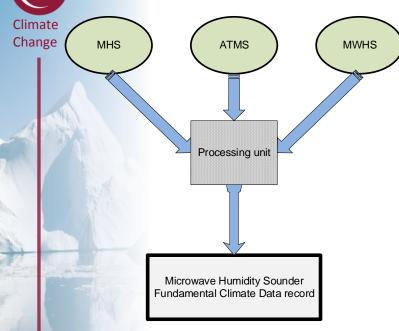
The processing unit applies the **measurement** equation to the measurement counts, propagates single effects to the uncertainty estimates, and records issues, represented by quality bit flags.
