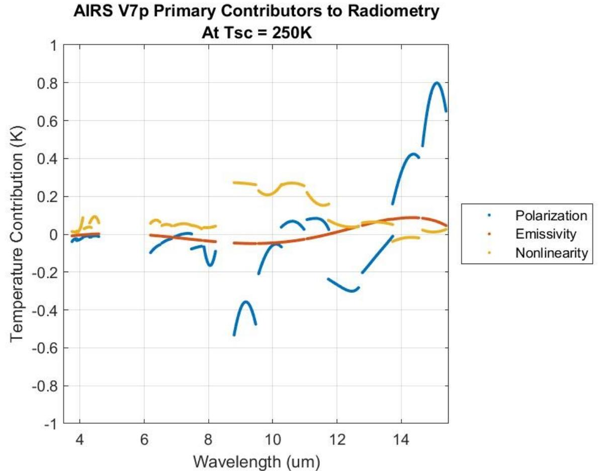
V7 Updates Polarization, Nonlinearity, Emissivity. First update to AIRS radiometry since launch
