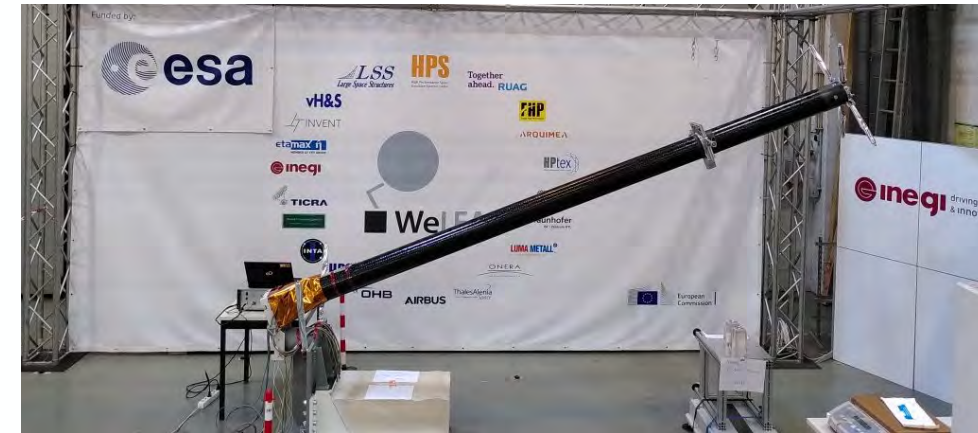
↑ Antenna boom during deployment testing. © HPS GmbH
