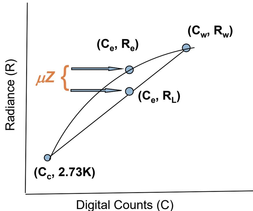
Schematic view of calibration equation
