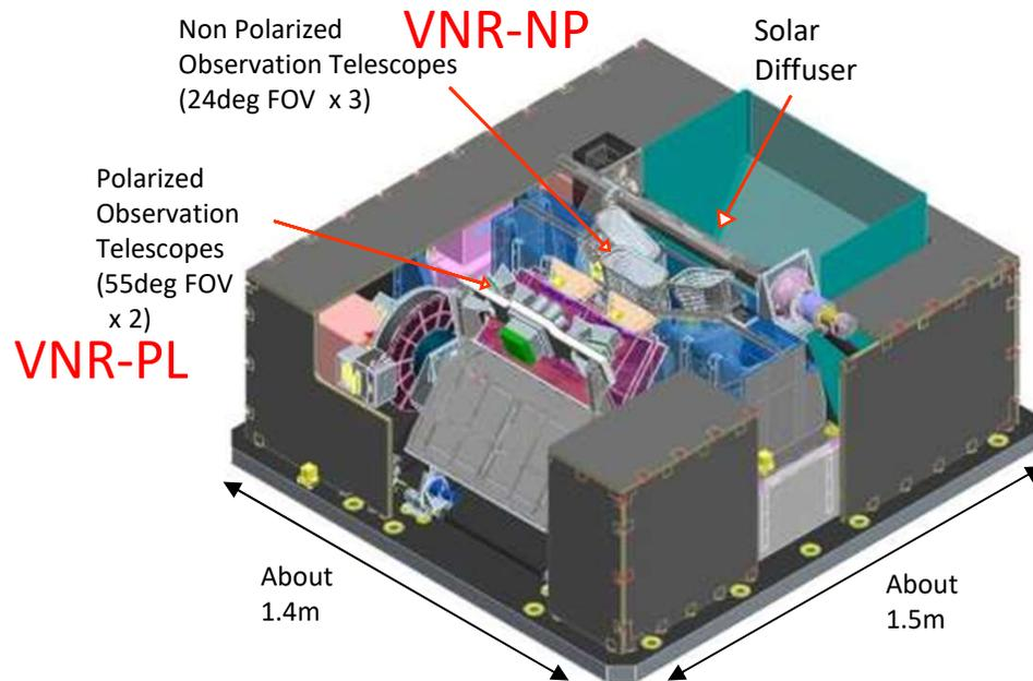
Visible and Near Infrared Radiometer
