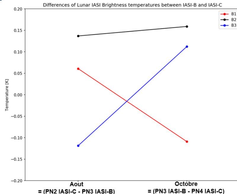
Difference of Lunar IASI Brightness Temperature between IASI-B and IASI-C in K
