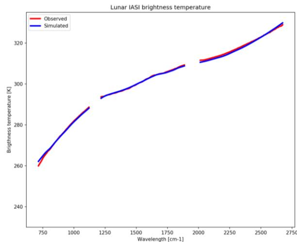
❖ The Moon is covering only a part of IASI pixel, so the non-linearity conversion in brightness temperature induce a different temperature for the 3 bands:
