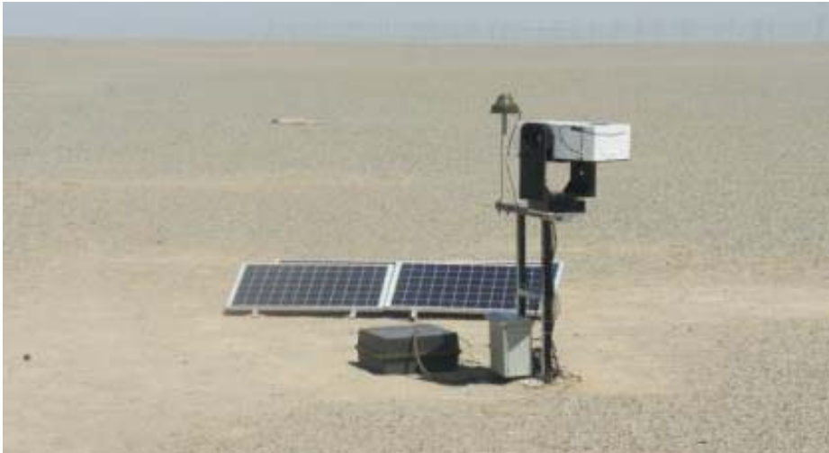
Atmosphere-Land reflectance spectral radiometer
