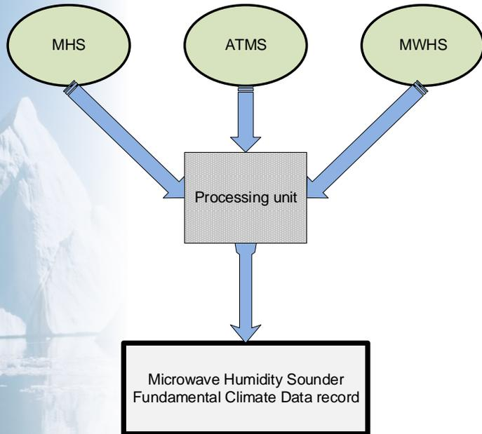
The processing unit applies the **measurement equation** to the measurement counts, propagates single effects to the **uncertainty estimates**, and records issues, represented by **quality bit flags**.
