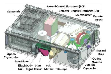
CIRAS provides accurate profiles of atmospheric temperature and water vapor in a 4U form factor
