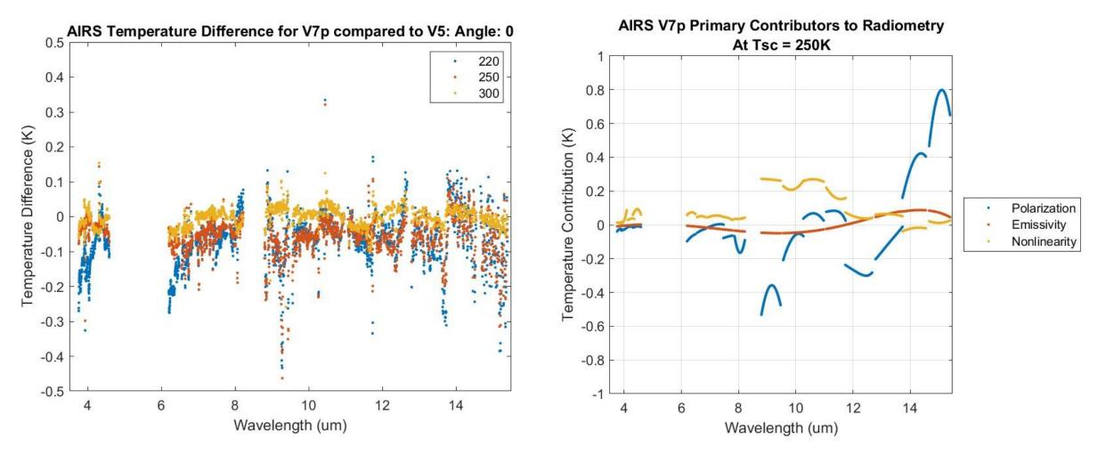
V7 Updates Polarization, Nonlinearity, Emissivity. First update to AIRS radiometry since launch
