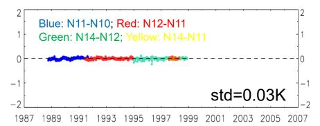
Global ocean mean inter-satellite difference time series (K) for MSU channel 2 onboard NOAA-10 to NOAA-14 (plot from Zou et al. 2009)
