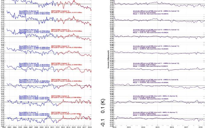
Left: Anomaly time series of Aqua/AMSU-A (blue) and S-NPP/ATMS (red) Observation Right: Their difference time series. Radiometric stability achieves 0.004K/Year for most (plot from Zou et al. 2018).
