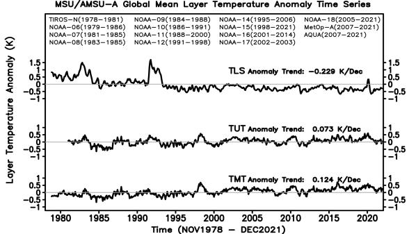
Mean Layer Temperatures Time Series for Mid-troposphere (TMT), Upper-Troposphere (TUT), and Lower-Stratosphere
