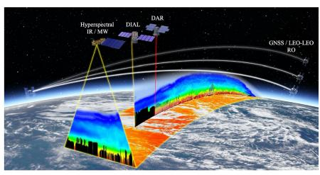
Hyperspectral Microwave sensors are listed as an *Essential Component* of the potential future global PBL observing system, to provide improved PBL and free tropospheric 3D temperature and water vapor structure context to active sensors (*e.g.*, lidars, radars) and in conjunction with other passive sensors (*e.g.*, infrared, radio-occultation).
