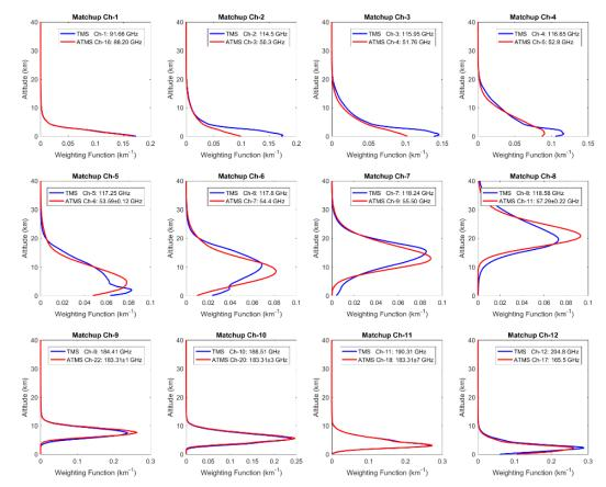
• A subset of ATMS channels that match up with TMS is used in retrieval, which permits a more direct comparison of the information content available between the V-band and F-band
