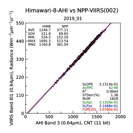
The gain calculated here can be used to convert a HIM8 count into a radiance, using the regression forced through the published visible space count of 20
