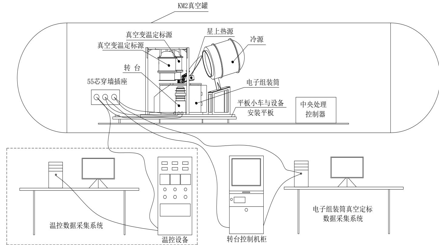
The receiver is placed inside the KM2 vacuum tank. The temperature is controlled externally and the turntable rotates. Temperature control data and electronic assembly cylinder data are collected for experimental analysis.
